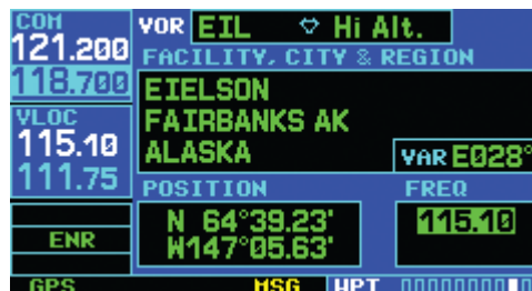
Figure 7-36 Activate the Standby Frequency
