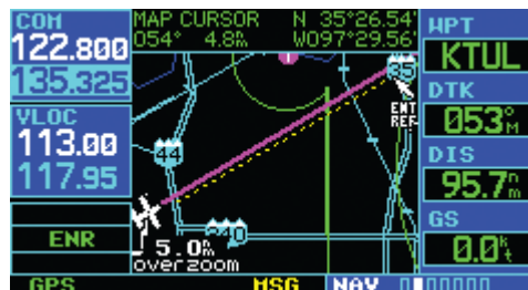
Figure 3-21 Using Pointer to Measure Distance and Bearing
