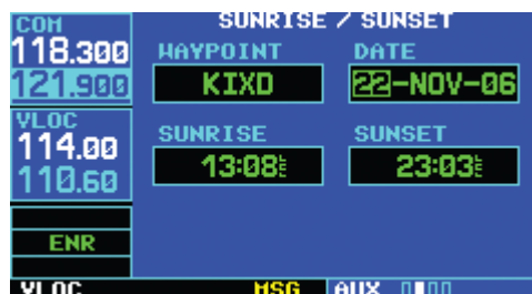
Figure 10-46 Date Field Highlighted
